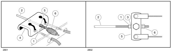
Figure 6-15 Rear Equalizer Adjustment
