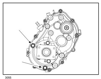
Figure 26-2 Lubricant Level Plug and Drain Plug
