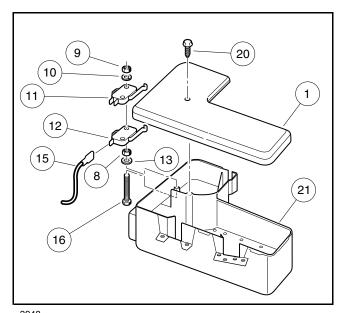
Figure 20-17 Accelerator Starter and Kill Limit Switches
