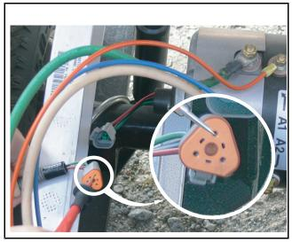
Figure 12-11 Test 13: Speed Sensor Black/White Wire
