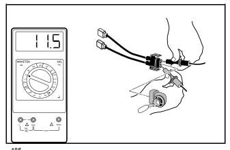
Figure 18-25 Voltage Measurement at Headlight Socket
