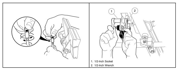
Figure 5-15 Brake Rod Adjustment
