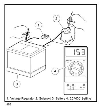
Figure 18-18 Voltage Regulator Test
