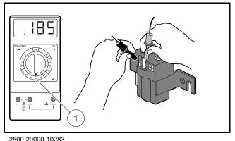
Figure 12-10 Activating Coil Test – Service Replacement Solenoid
