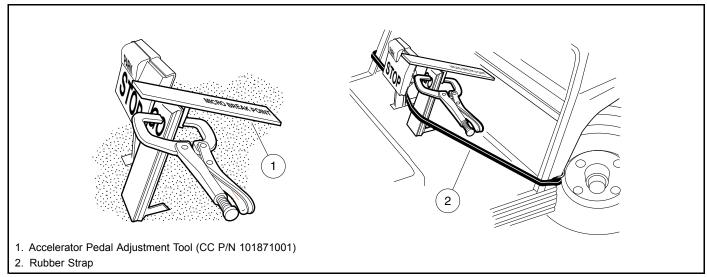
Figure 5-27 Accelerator Pedal Height Adjustment
