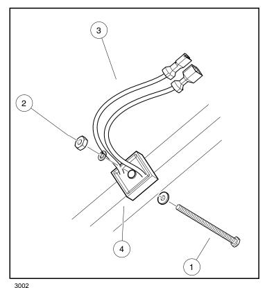
Figure 20-20 Voltage Limiter
