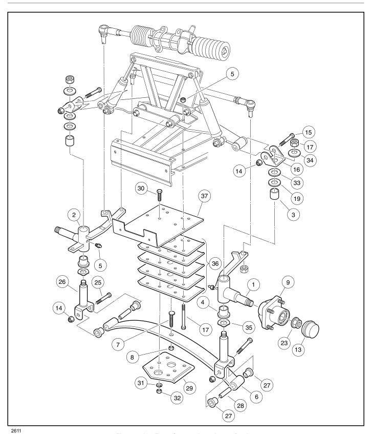
Figure 7-19 Front Suspension – Lower Portion
