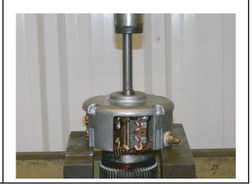
Figure 16-7 Armature Removal
