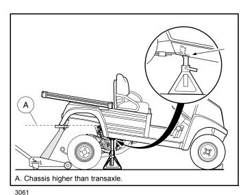
Figure 26-10 Raise Vehicle and Support On Jack Stands
