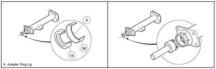
Figure 17-3 Axle Seal and Adapter Ring
