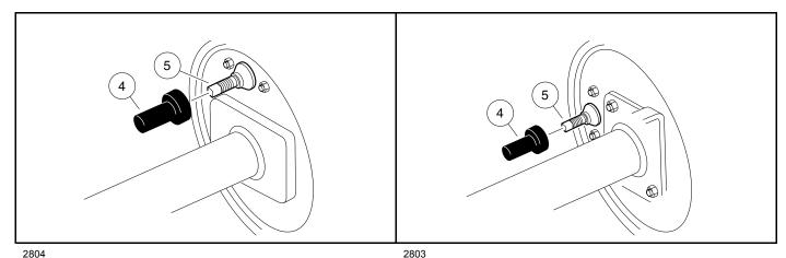
Figure 6-17 Rear Brake Adjustment Bolt
