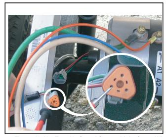
Figure 12-13 Test 13: Speed Sensor Light Green Wire
