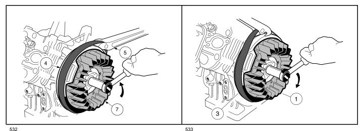
Figure 22-9 Flywheel Nut Removal
