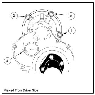
Figure 16-21 Motor Tightening Sequence
