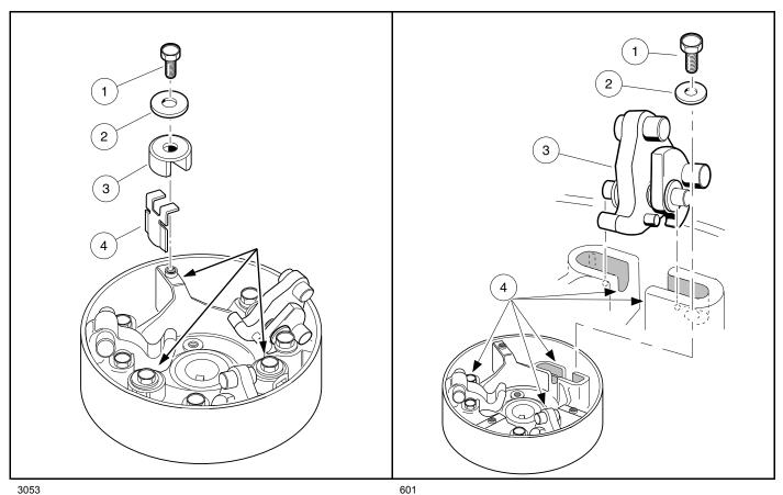
Figure 25-8 Drive Button Mounting
