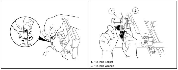
Figure 5-25 Brake Rod Adjustment
