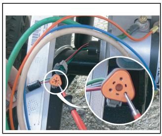
Figure 12-12 Test 13: Speed Sensor Red Wire
