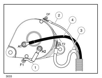
Figure 20-13 Starter/Generator Wiring
