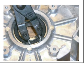
Figure 16-8 Brush Rigging Removal
