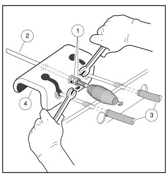
Figure 5-9 Loosen Rear Brake Equalizer Rod Nuts
