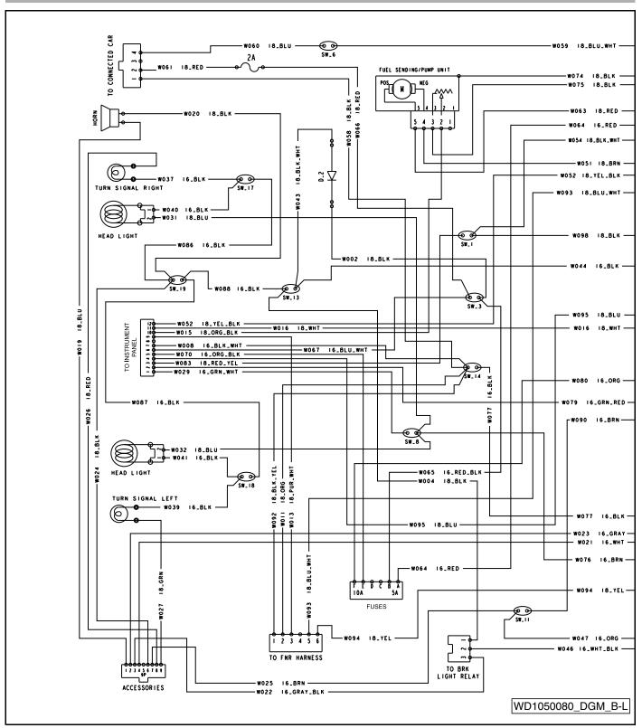
Figure 19-1 Wiring Diagram for Key-Start Gasoline Vehicle
