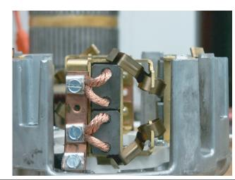
Figure 16-6 Brush Springs Positioning
