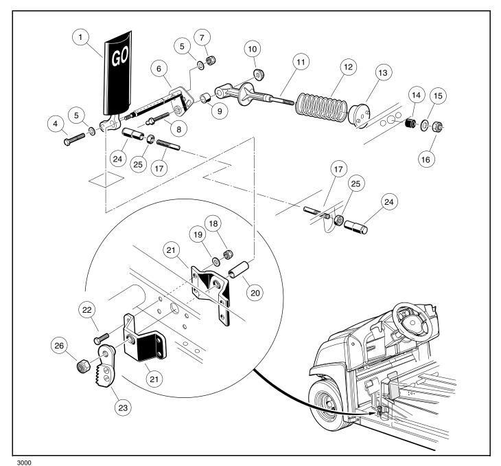
Figure 5-6 Accelerator Pedal – Gasoline Vehicles
