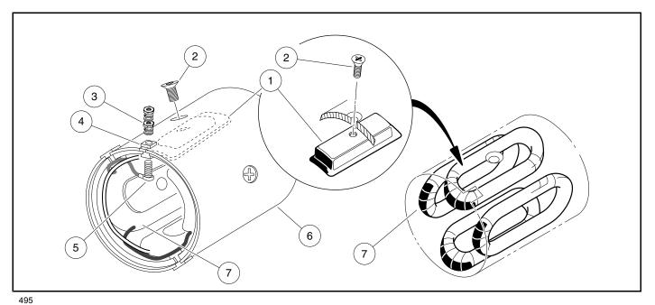
Figure 20-9 Field Coil Assembly
