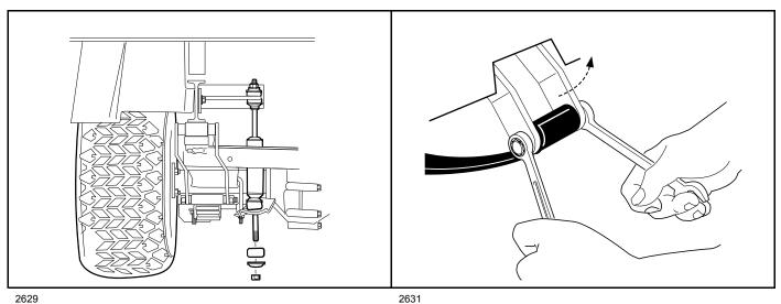
Figure 17-8 Disconnect Shocks
