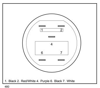
Figure 18-22 Fuel Gauge/Hour Meter
