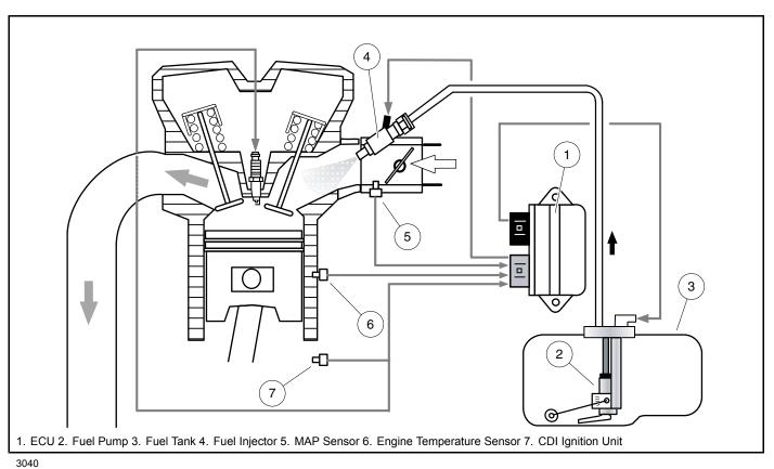
Figure 23-1 EFI System Components
