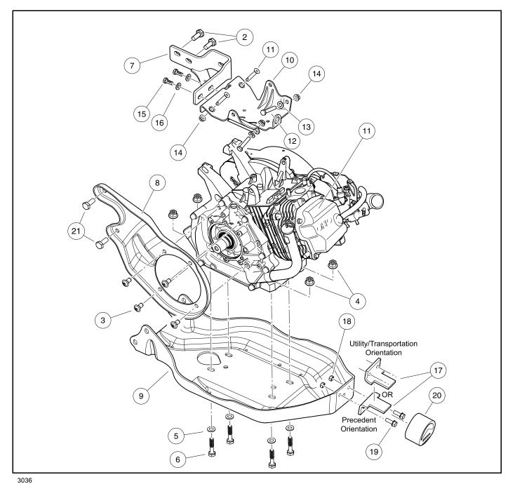
Figure 22-7 EX40 Engine and Mounting Brackets
