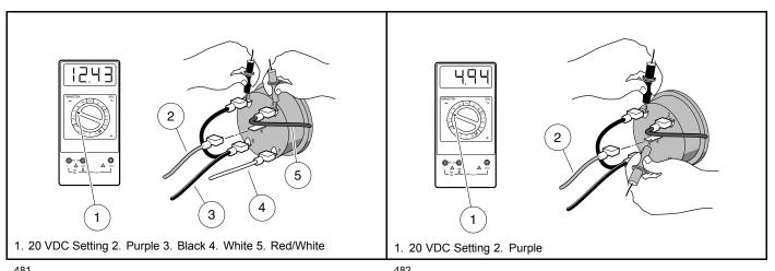
Figure 18-23 Fuel Gauge Voltage Test - Terminal 2
