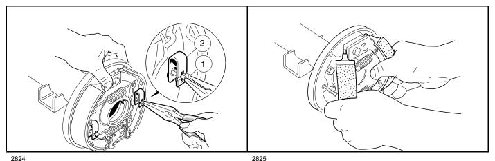
Figure 6-3 Rotate Clip Retainer
