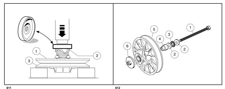
Figure 25-17 Cam Press Tool
