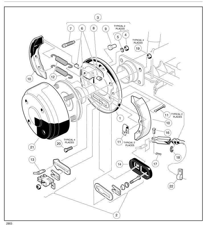
Figure 6-20 Rear Manually-Adjusted Brake Assembly
