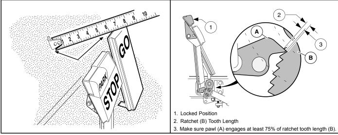
Figure 5-13 Accelerator Pedal Height Measurement
