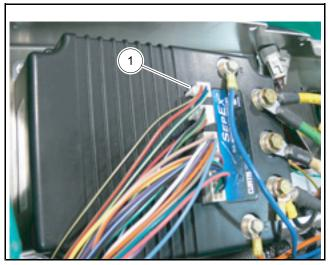
Figure 11-3 Disconnect Four-pin Connector.
