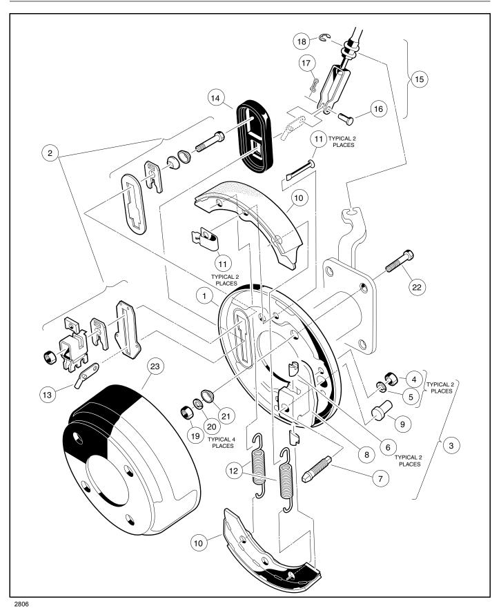
Figure 6-19 Front Manually Adjusted Brake Assembly
