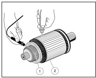
Figure 16-10 Armature Test
