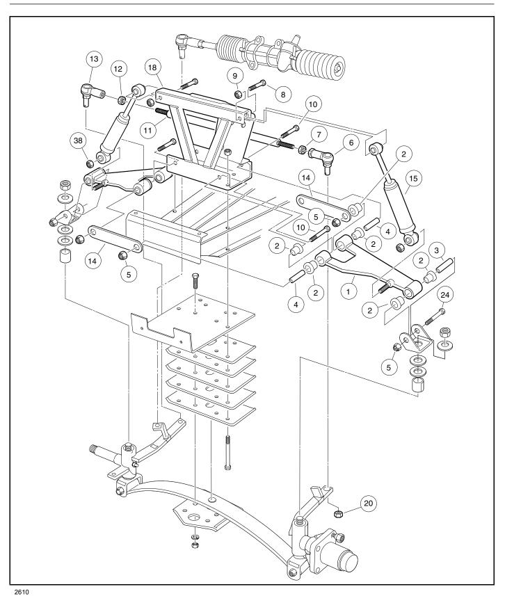
Figure 7-18 Front Suspension – Upper Portion
