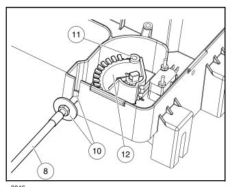
Figure 23-10 Accelerator Cable At Electrical Component
