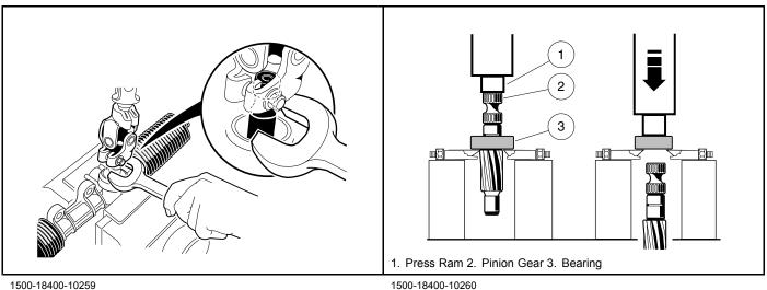
Figure 7-7 Remove Pinion from Housing
