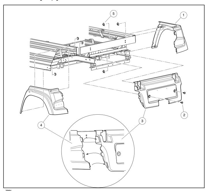
Figure 4-8 Rear Fender and Tailskirt
