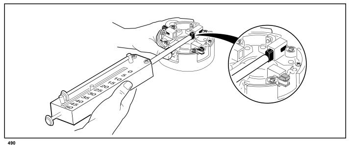
Figure 20-4 Brush Spring Tension Test
