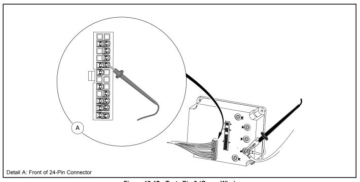
Figure 12-17 Test: Pin 8 (Green Wire)
