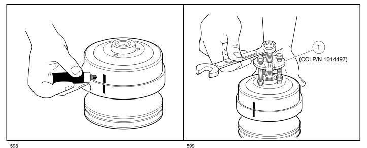
Figure 25-6 Mark Drive Clutch Hub
