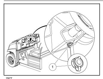
Figure 11-2 Communication Port Under Instrument Panel
