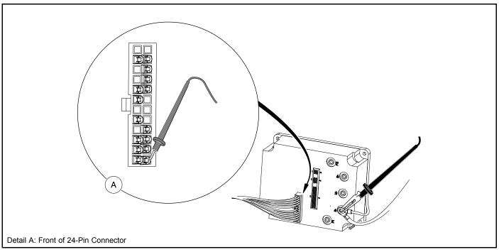
Figure 12-20 Test: Pin 1 (Tan Wire)
