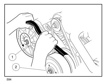
Figure 25-2 Drive Belt Removal
