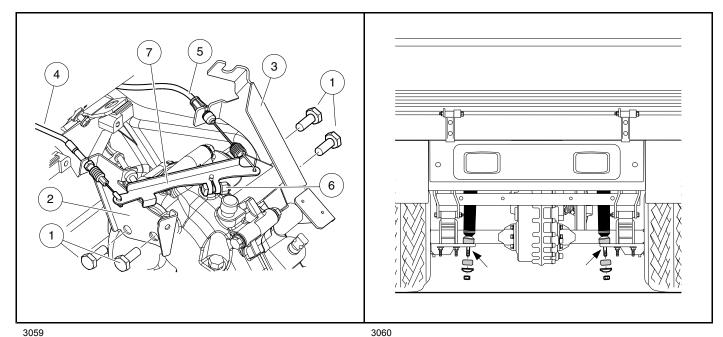
Figure 26-6 Governor Arm, Cable and Brackets
