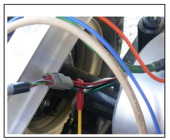
Figure 12-14 Test 13: Speed Sensor Green Wire
