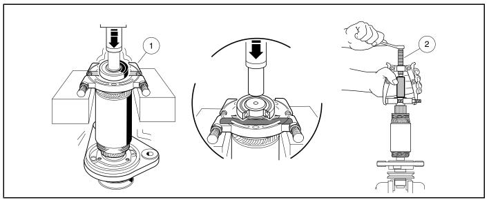
Figure 20-8 Bearing Removal
