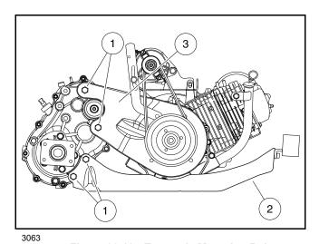
Figure 26-12 Transaxle Mounting Bolts
