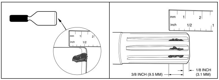
Figure 16-17 Grease on Putty Knife
