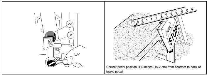
Figure 5-10 Brake Pedal Height Adjustment
