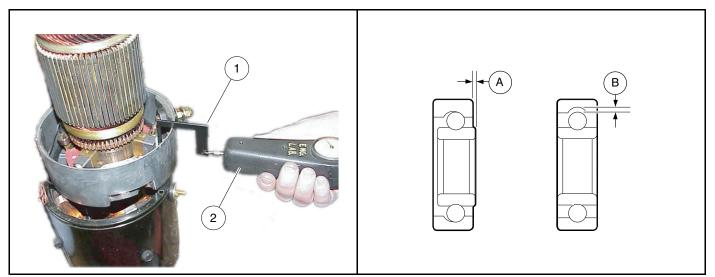
Figure 16-11 Brush Spring Tension Test
