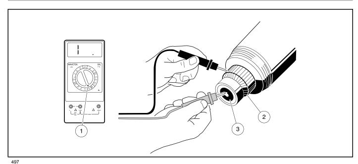
Figure 20-11 Armature Ground Test
