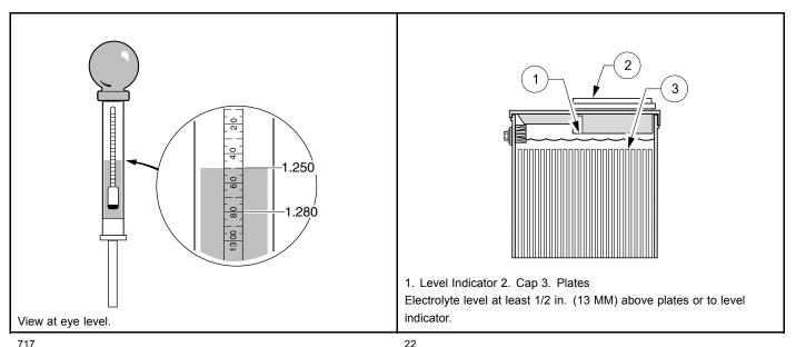
Figure 18-7 Hydrometer Test
