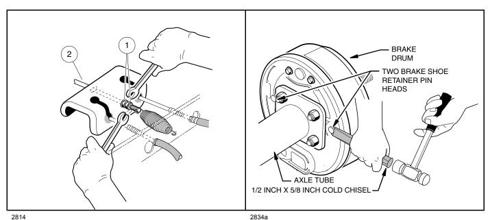
Figure 6-1 Loosen Equalizer Nut
