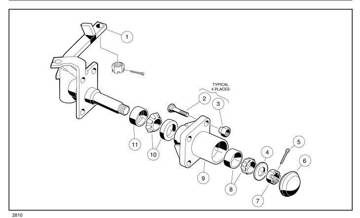
Figure 6-22 Front Spindle Assembly
