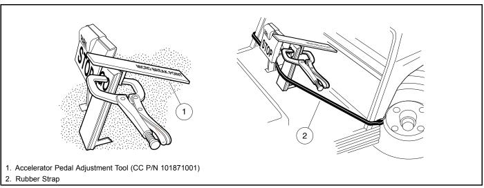
Figure 5-17 Accelerator Pedal Height Adjustment
