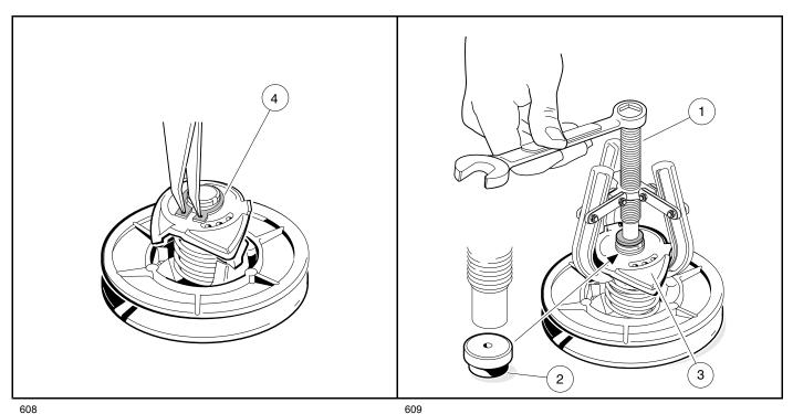
Figure 25-15 Remove Retaining Ring
