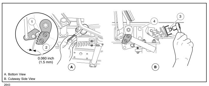
Figure 5-22 Park Brake Ratchet/Pawl Gap Adjustment
