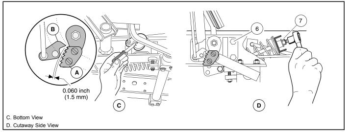
Figure 5-12 Park Brake Ratchet/Pawl Gap Adjustment
