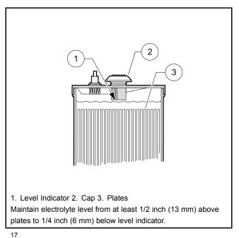
Figure 14-3 Electric Battery Electrolyte Level
