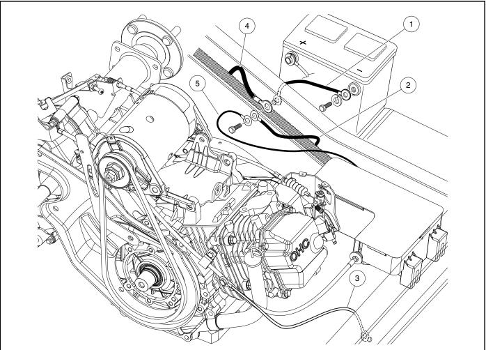
1. Battery Ground 2. Main Wire Harness Ground 3. Engine Ground Cable 4. Starter/Generator Ground (from A1 Terminal) 5. Voltage Regulator Ground Wire (from electrical component box)
