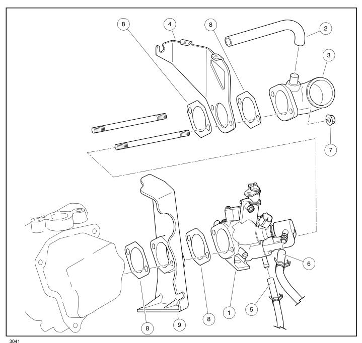
Figure 23-2 Throttle Body - Exploded View
