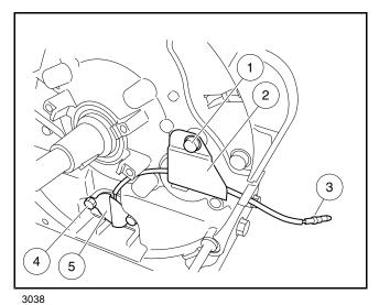
Figure 22-11 Oil Level Sensor - EX40
