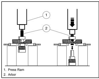
Figure 17-13 Intermediate Gear Assembly
