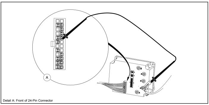
Figure 12-18 Test: Pin 19 (Orange/White Wire)
