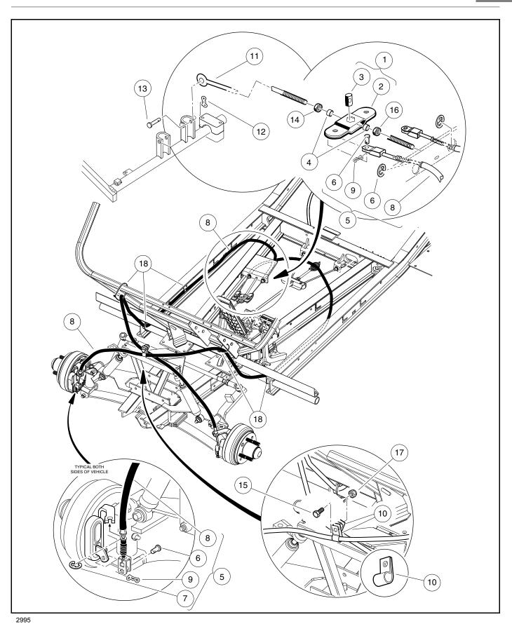
Figure 6-23 Front Brake Cables and Equalizer
