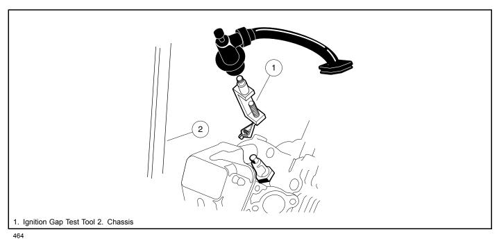
Figure 18-20 Ignition Spark Test
