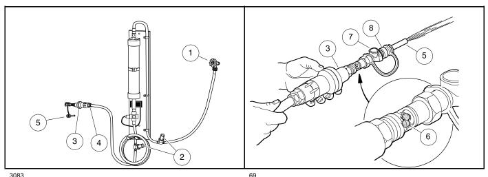
Figure 14-4 Connecting Hose with Filter to Water Source
