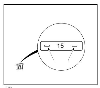
Figure 18-9 Testing the ATC and ATM-style Blade Fuse
