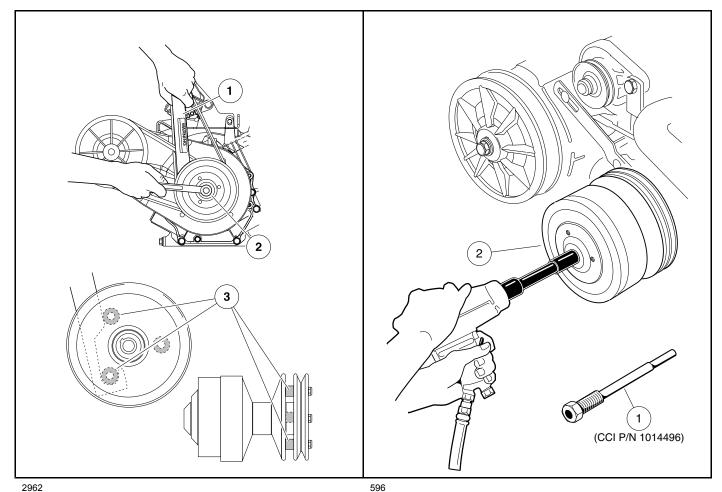
Figure 25-4 Loosen Retaining Bolt
