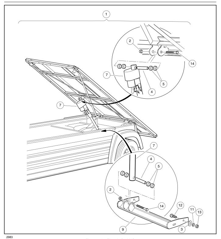
Figure 4-9 Electric Bed Lift
