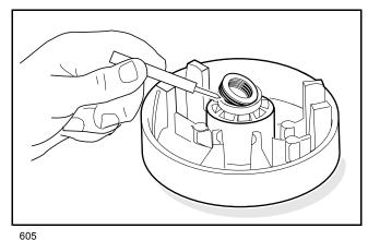
Figure 25-11 Spiral Back-up Rings
