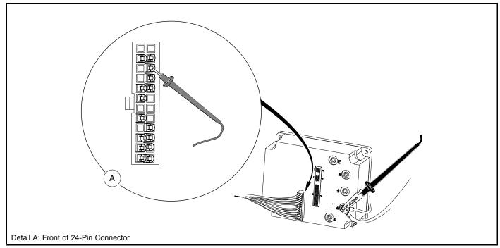
Figure 12-19 Test: Pin 10 (Black Wires)
