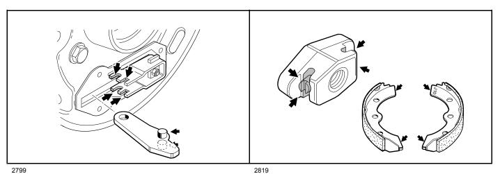
Figure 6-9 Lubricate Actuator
