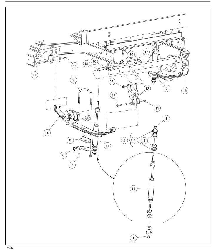
Figure 9-4 Rear Suspension Assembly and Mounting
