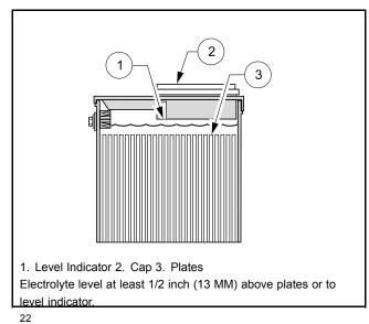
Figure 20-22 Battery Electrolyte Level
