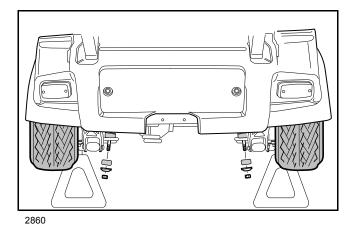
Figure 9-1 Shock Absorber Removal
