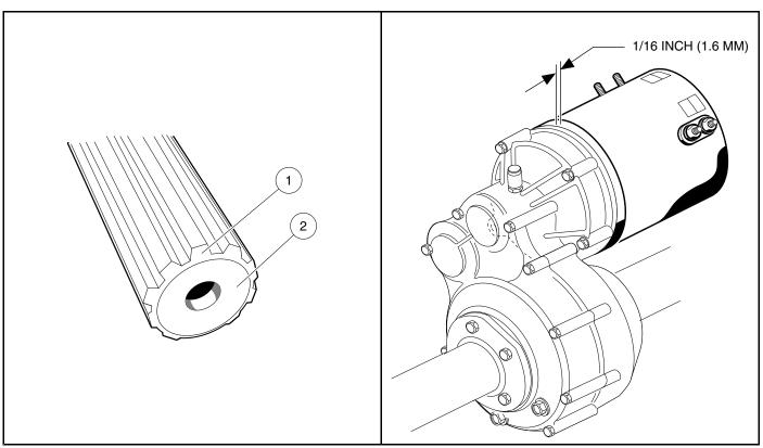
Figure 16-19 Clean Chamfer and Input Shaft End
