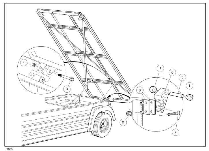
Figure 4-10 Electric Bed Mounting
