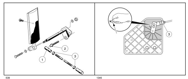
Figure 23-4 Accelerator Rod
