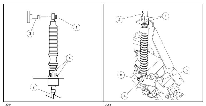
Figure 26-13 Shifter Cable at FNR Handle
