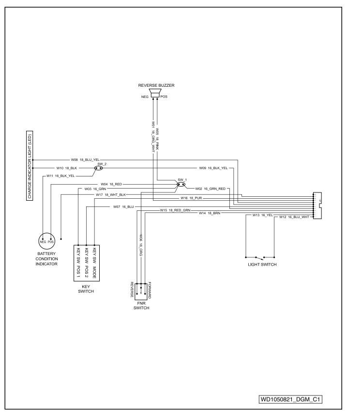
Figure 12-3 Wiring Diagram – Instrument Panel
