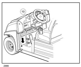
Figure 5-2 Brake Pedal Weldment Through Floor
