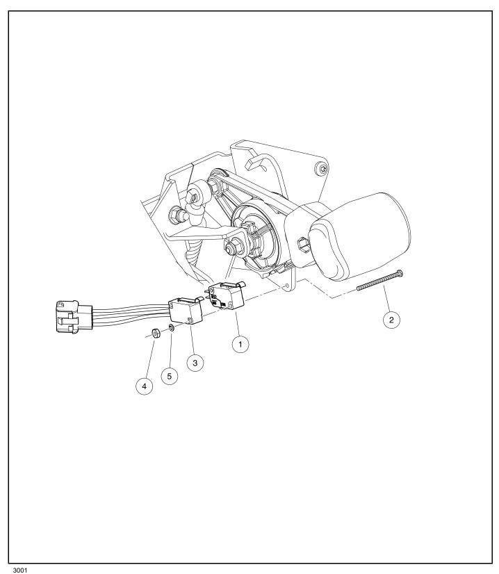
Figure 20-19 Forward/Reverse Assembly Switches
