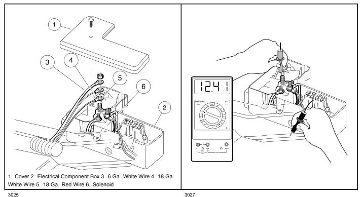
Figure 18-12 Solenoid Wire Removal
