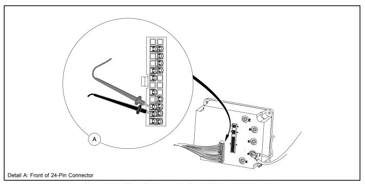
Figure 12-16 Test: Pins 14 and 15 (Purple/White and Yellow wires)
