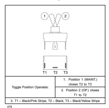
Figure 18-14 Maintenance/Operate Switch Test – for Pedal-Start Vehicles
