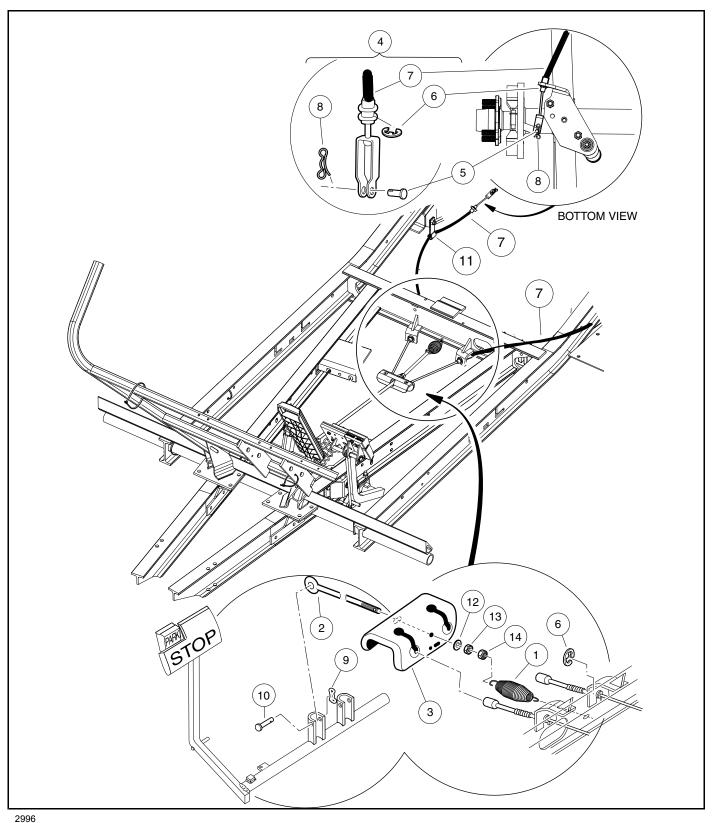
Figure 6-24 Rear Brake Cables and Equalizer
