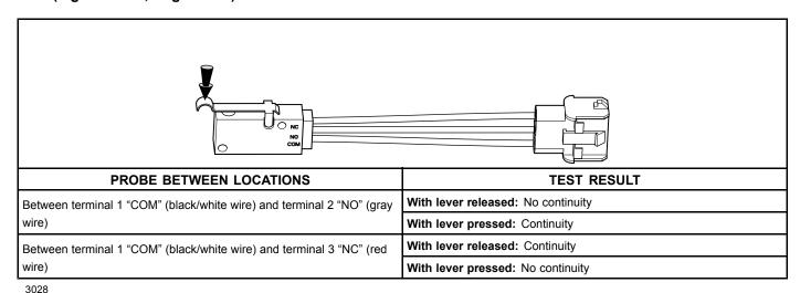
Figure 18-15 Neutral Lockout Limit Switch Test
