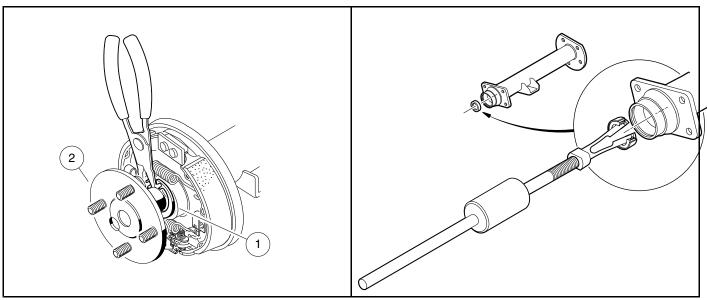
Figure 17-1 Remove Internal Retaining Ring
