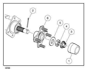
Figure 26-3 Rear Hub Exploded View
