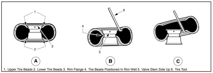
Figure 8-1 Tire Removal
