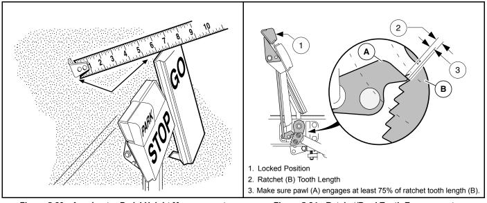
Figure 5-23 Accelerator Pedal Height Measurement
