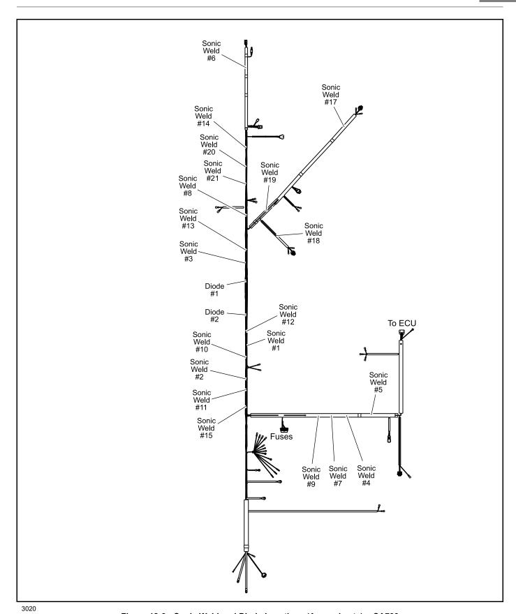
Figure 18-6 Sonic Weld and Diode Locations (Approximate) - CA700
