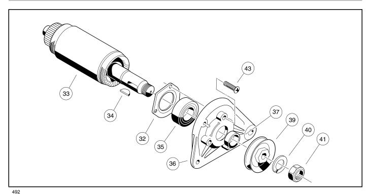
Figure 20-6 Armature and Output End Cover Assembly
