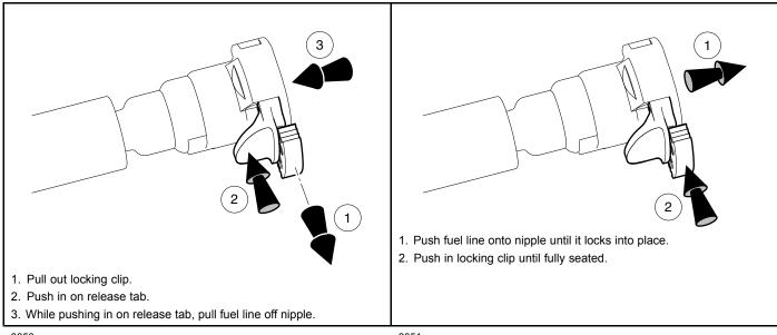
Figure 23-13 Fuel Line Connector - To Disconnect
