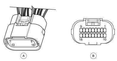
18-PIN CONNECTOR (GRAY AND BLACK): A. ECU SIDE OF CONNECTOR B. WIRE ENTRY SIDE OF CONNECTOR
