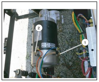
Figure 12-15 Test A1 and A2 Motor Voltage
