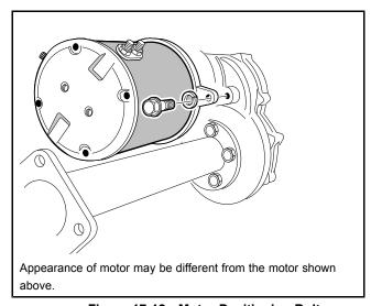
Figure 17-12 Motor Positioning Bolt
