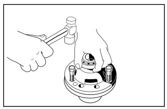
Figure 17-14 Separate Housing
