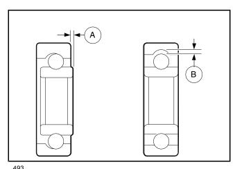
Figure 20-7 Bearing Play Inspection
