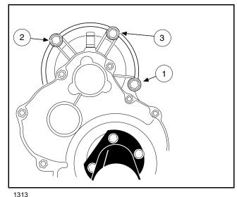
Figure 16-25 EJ8–4001A Motor Mounting Bolts and Tightening Sequence
