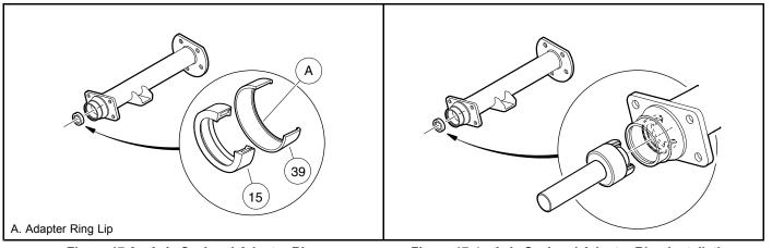
Figure 17-3 Axle Seal and Adapter Ring
