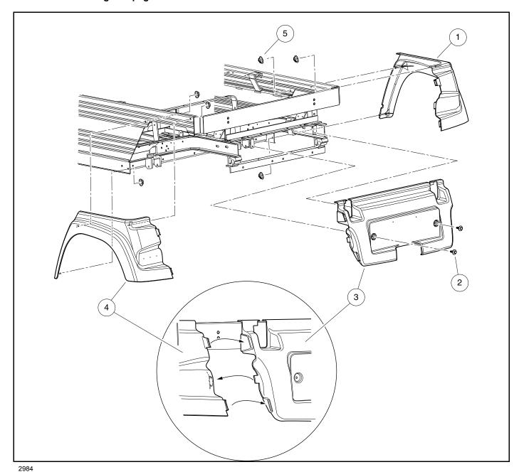
Figure 4-8 Rear Fender and Tailskirt
