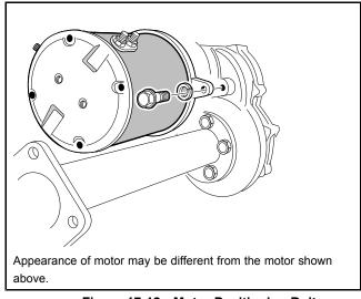
Figure 17-12 Motor Positioning Bolt
