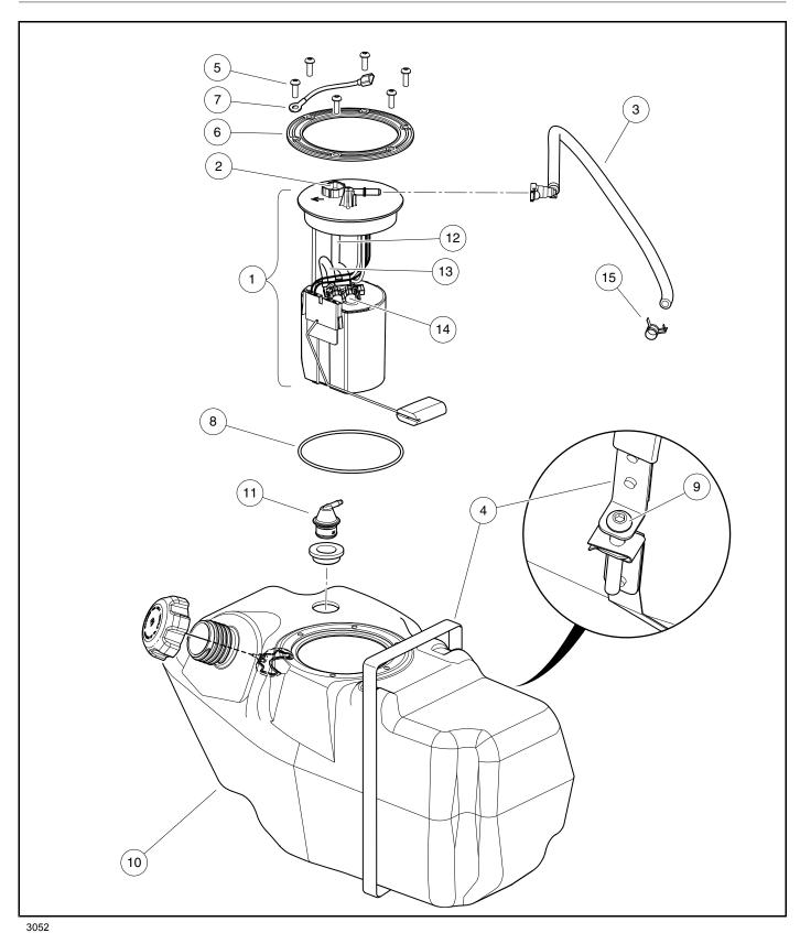
Figure 23-15 Fuel System (Side-Fill) – Exploded View
