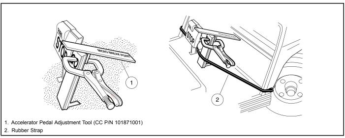
Figure 5-27 Accelerator Pedal Height Adjustment
