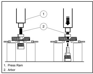
Figure 17-13 Intermediate Gear Assembly
