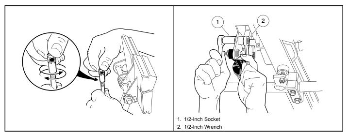
Figure 5-15 Brake Rod Adjustment
