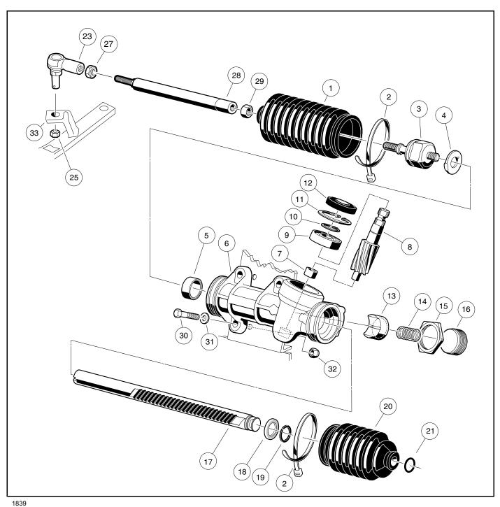
Figure 7-10 Steering Gear - Maintenance-Free Ball Joints
