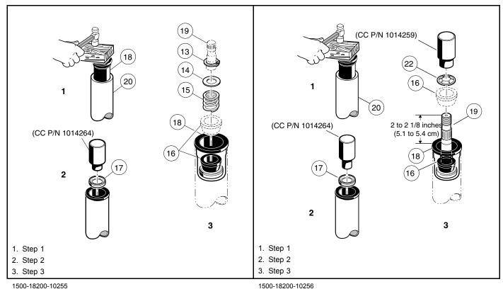
Figure 7-4 Steering Shaft – Bottom End
