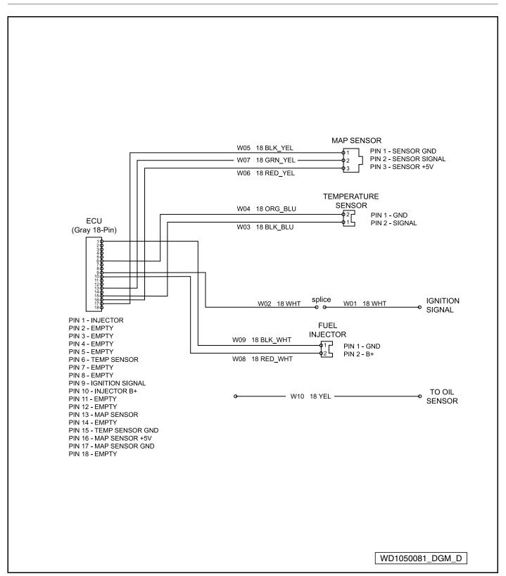
Figure 19-4 Wiring Diagram – EFI and Engine
