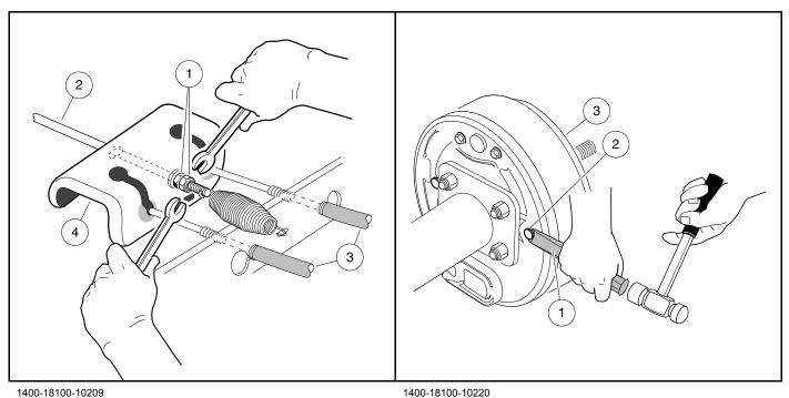
Figure 6-1 Loosen Brake Cables
