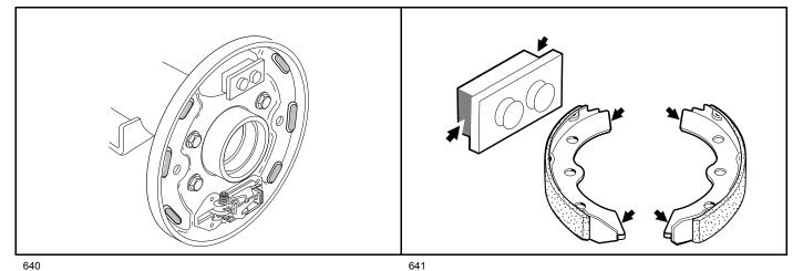
Figure 6-8 Apply Grease On Bosses
