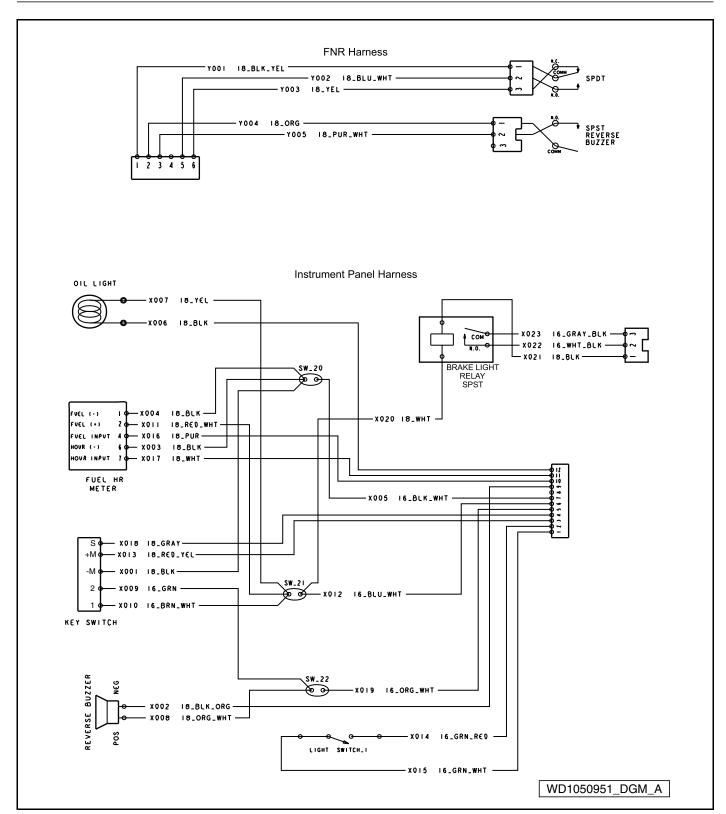
Figure 18-3 Wiring Diagram - Instrument Panel and FNR Shifter
