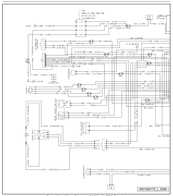
Figure 12-1 Wiring Diagram - CA300 with ERIC Charging
