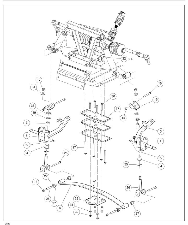
Figure 7-19 Front Suspension – Lower Portion
