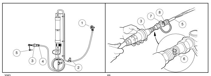
Figure 14-5 Connecting Hose with Filter to Water Source
