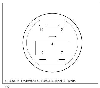
Figure 18-19 Fuel Gauge/Hour Meter
