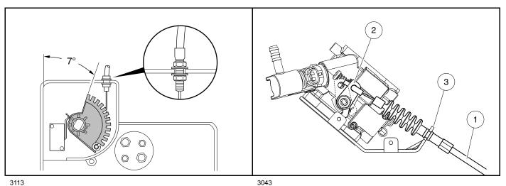
Figure 23-6 Accelerator Cable Cam Position – 7° (Top View)
