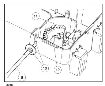
Figure 23-10 Accelerator Cable At Electrical Component Box
