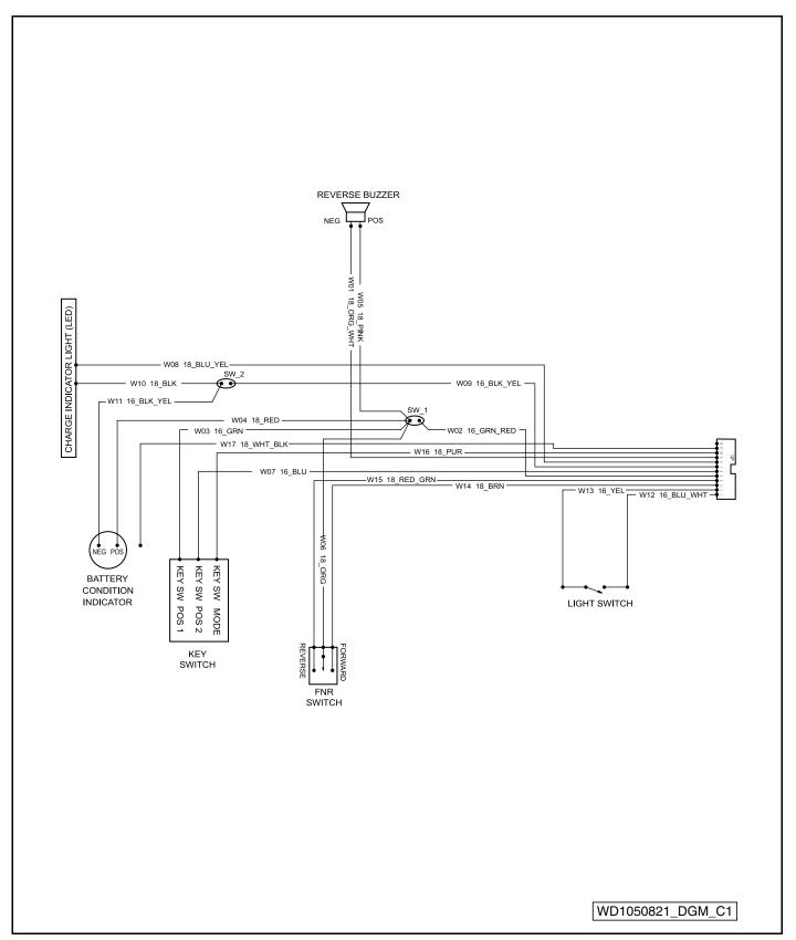
Figure 12-3 Wiring Diagram – Instrument Panel
