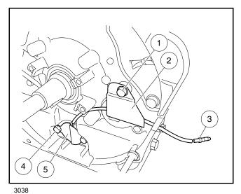
Figure 22-11 Oil Level Sensor - EX40
