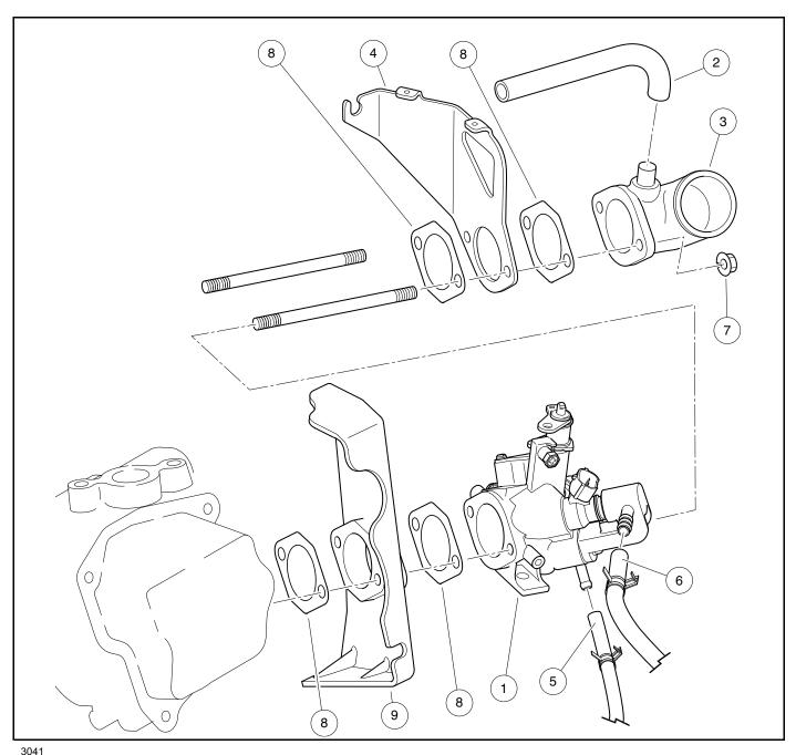
Figure 23-2 Throttle Body - Exploded View
