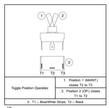
Figure 19-7 Maintenance/Operate Switch Test – for Key-Start Vehicles
