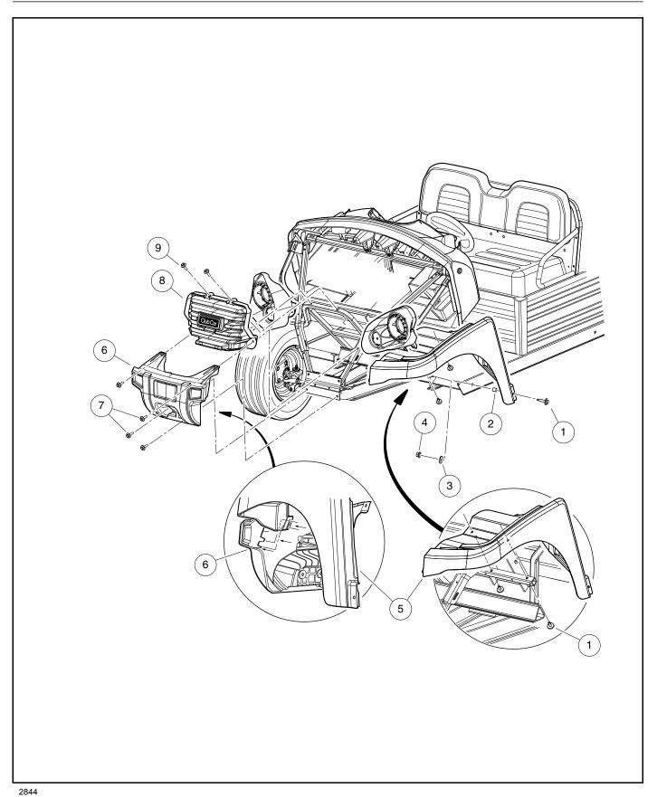
Figure 4-3 Front Grille, Bumper, and Side Fenders
