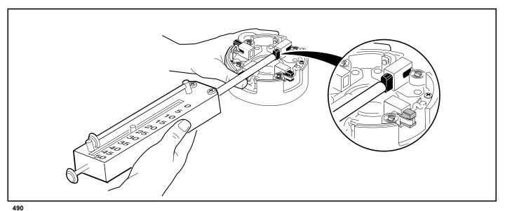
Figure 20-4 Brush Spring Tension Test
