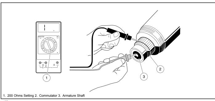
Figure 20-11 Armature Ground Test
