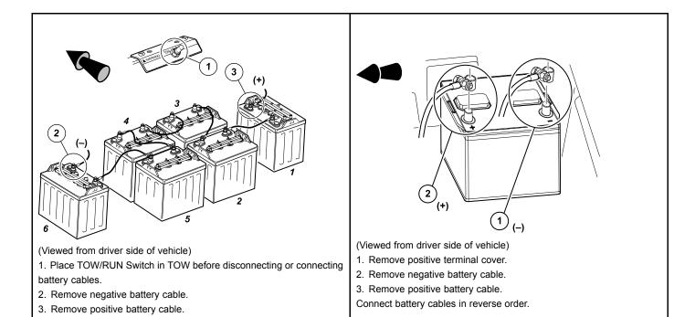
Figure 1-1 Battery Cable Removal- Electric Vehicle
