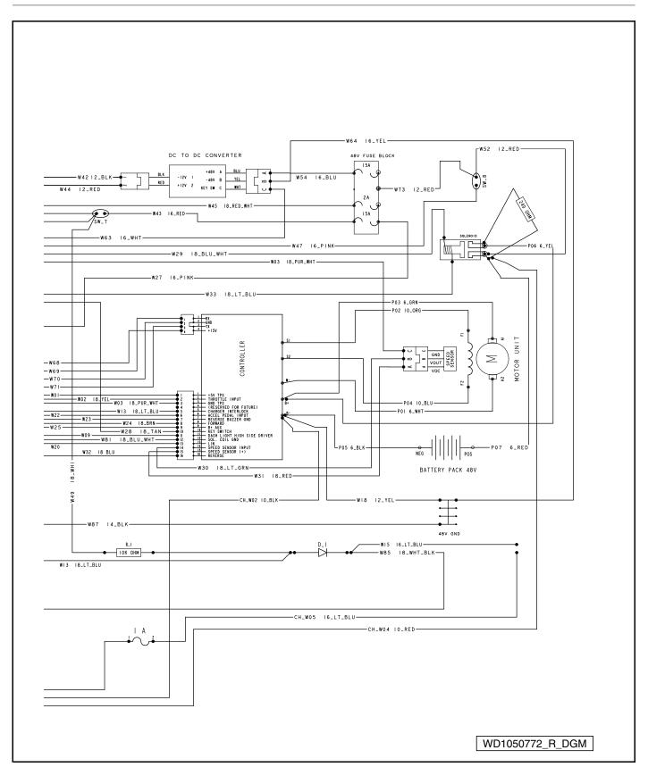
Figure 12-2 Wiring Diagram – CA300 with ERIC Charging (Continued)
