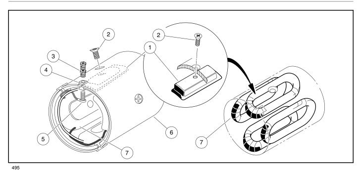
Figure 20-9 Field Coil Assembly
