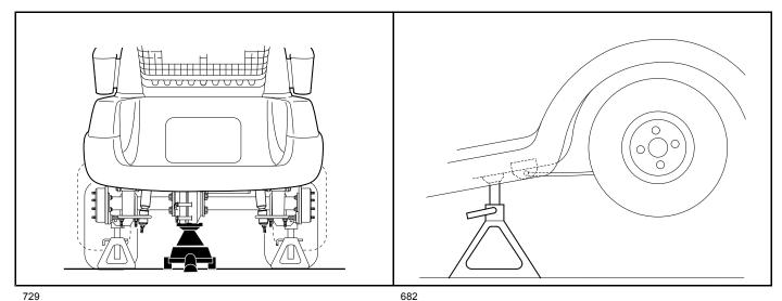
Figure 16-1 Lift Vehicle with Floor Jack
