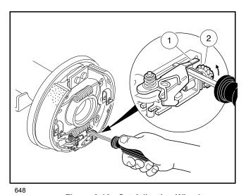
Figure 6-16 Set Adjusting Wheel
