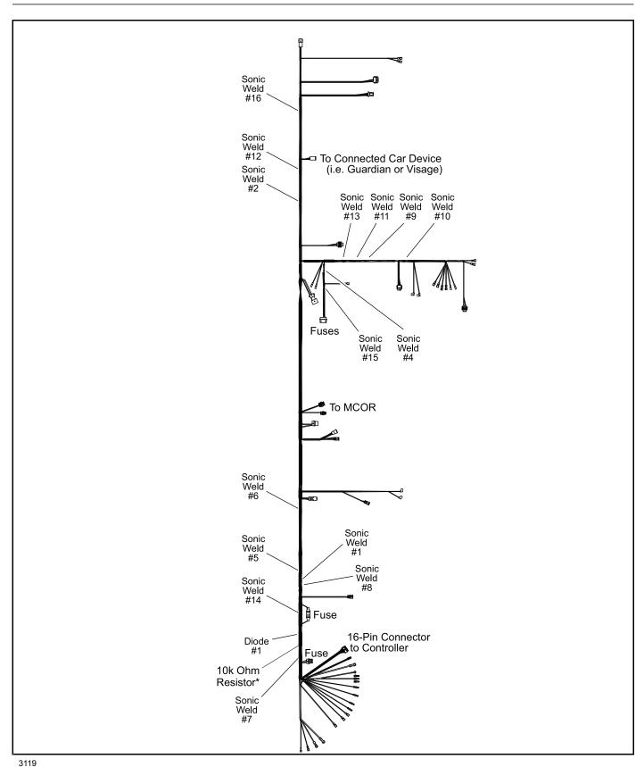
Figure 12-5 Sonic Weld, Diode and 10k Ohm Resistor Locations (Approximate) - CA300 with ERIC Charging
