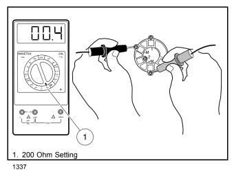
Figure 18-8 Key Switch Test – Engine Kill Circuit
