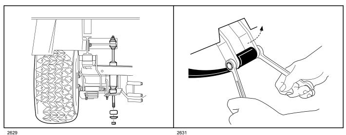
Figure 17-8 Disconnect Shocks
