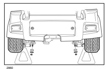
Figure 9-1 Shock Absorber Removal
