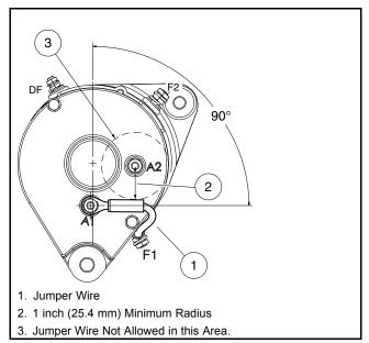
Figure 20-12 A1 to F1 Terminal Jumper Wire Routing
