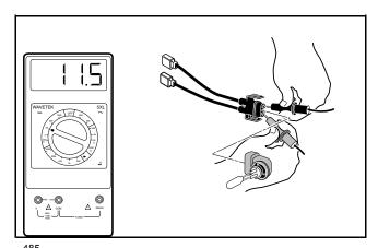
Figure 18-22 Voltage Measurement at Headlight Socket
