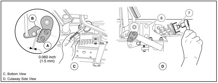
Figure 5-12 Park Brake Ratchet/Pawl Gap Adjustment
