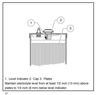
Figure 14-3 Electric Battery Electrolyte Level
