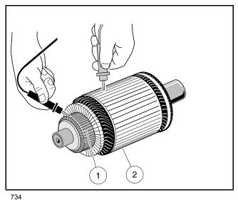
Figure 16-12 Armature Test
