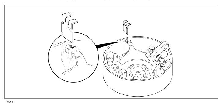
Figure 25-13 Correct Orientation of Drive Button Take-up Springs
