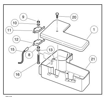
Figure 20-20 Accelerator Starter and Kill Limit Switches
