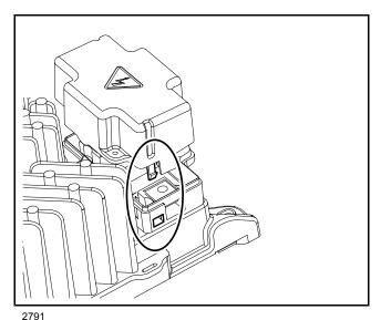
Figure 15-9 Terminal Block Cover Mounting Tabs
