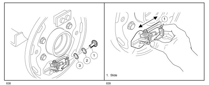
Figure 6-5 Remove Adjuster Wheel
