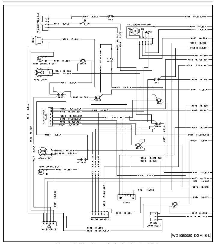
Figure 19-1 Wiring Diagram for Key-Start Gasoline Vehicle
