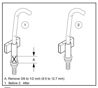
Figure 20-17 Belt Tension Tool Modification (If Necessary)
