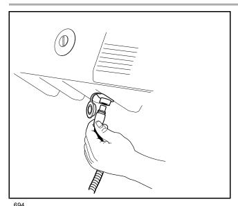
Figure 11-2 Communication Port Under Instrument Panel
