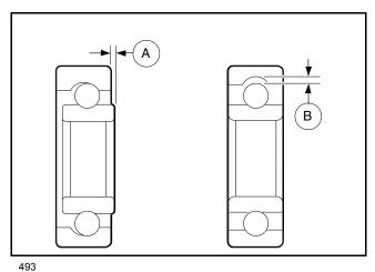
Figure 20-7 Bearing Play Inspection
