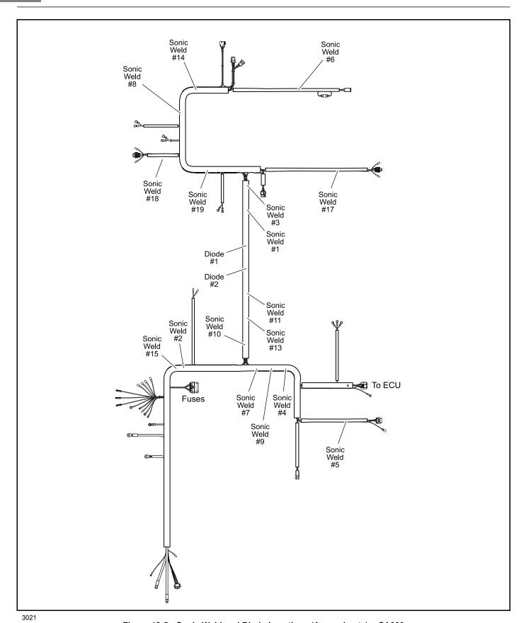
Figure 18-5 Sonic Weld and Diode Locations (Approximate) - CA300
