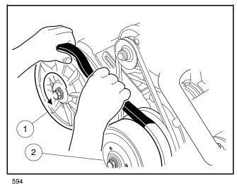
Figure 25-2 Drive Belt Removal
