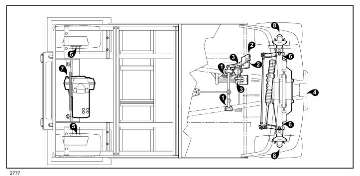
Figure 10-1 Lubrication Points – Electric Vehicles
