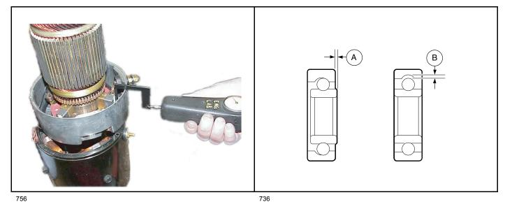
Figure 16-13 Brush Spring Tension Test
