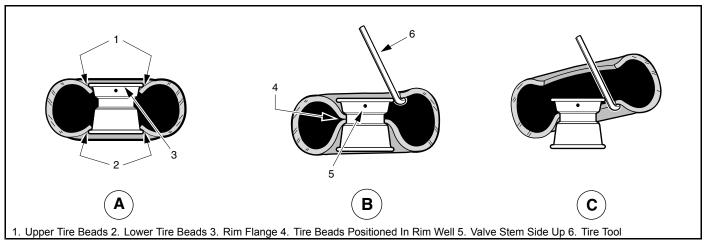
Figure 8-1 Tire Removal
