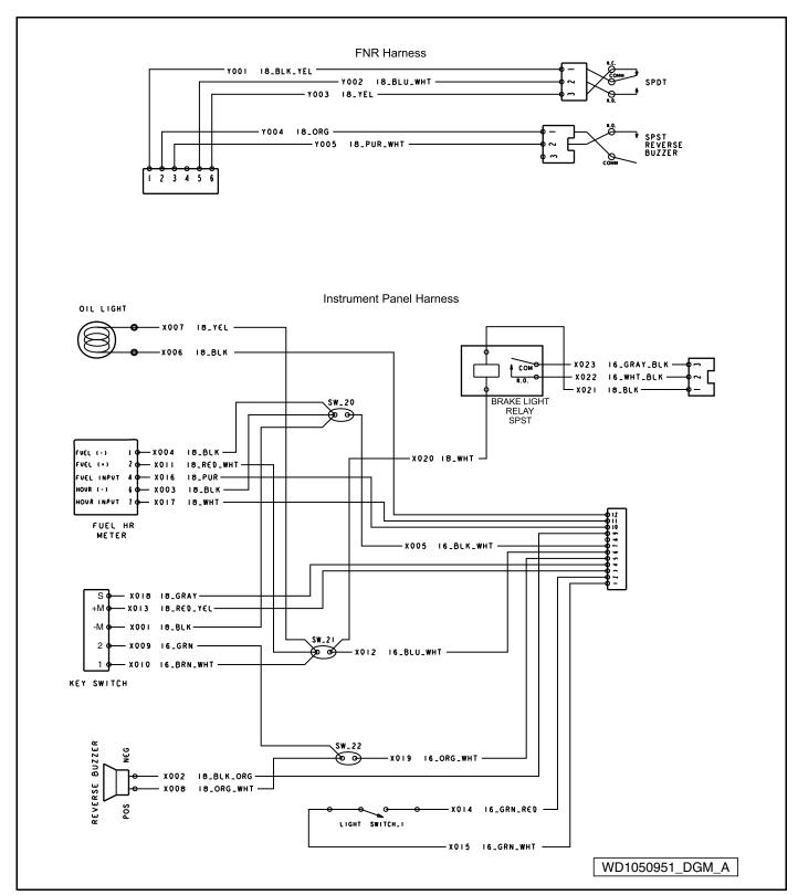
Figure 19-3 Wiring Diagram - Instrument Panel and FNR Shifter
