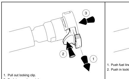
1. Push fuel line onto nipple until it locks into place. 2. Push in locking clip until fully seated.
