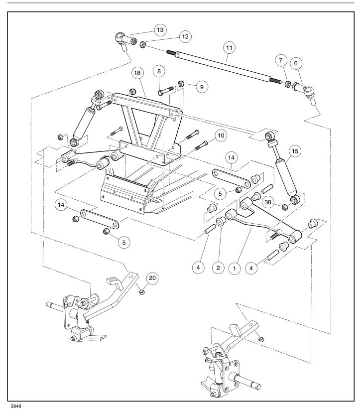
Figure 7-18 Front Suspension – Upper Portion
