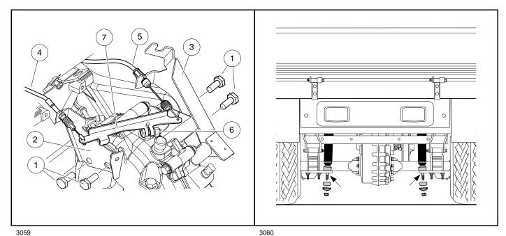
Figure 26-6 Governor Arm, Cable and Brackets
