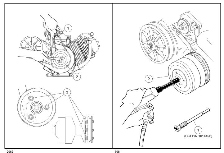
Figure 25-4 Loosen Retaining Bolt
