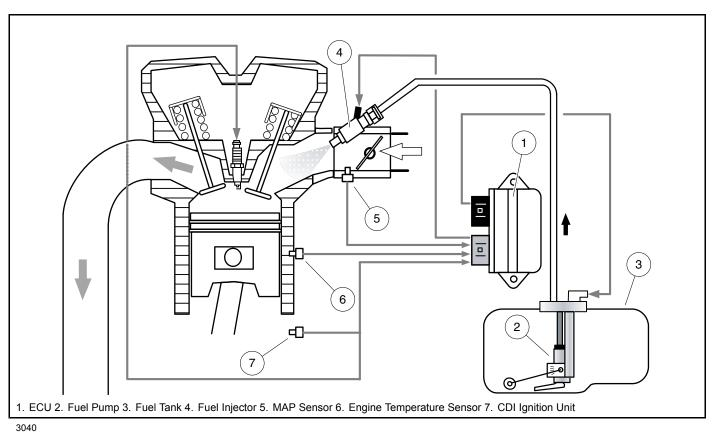
Figure 23-1 EFI System Components
