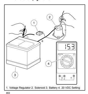
Figure 18-15 Voltage Regulator Test
