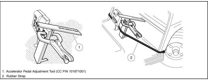
Figure 5-17 Accelerator Pedal Height Adjustment
