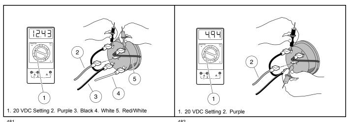
Figure 18-20 Fuel Gauge Voltage Test - Terminal 2
