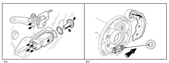
Figure 6-10 Apply Grease To Brake Adjuster
