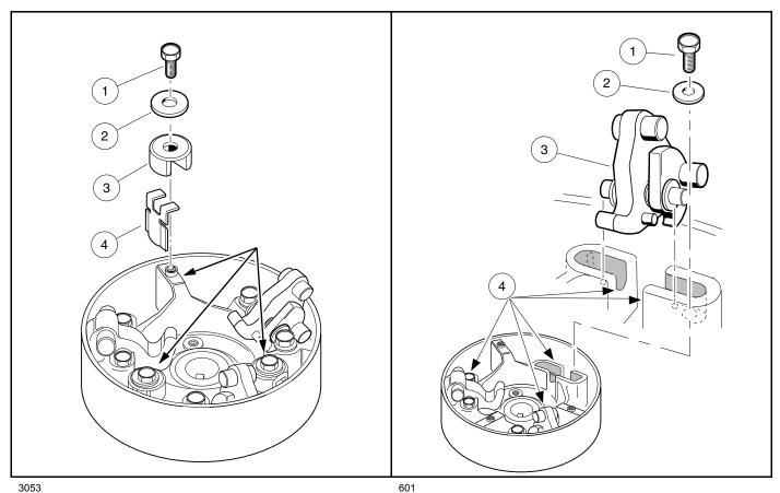
Figure 25-8 Drive Button Mounting
