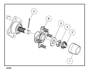
Figure 26-3 Rear Hub Exploded View
