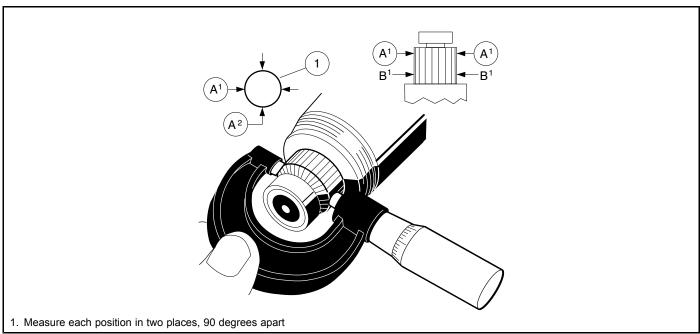
Figure 20-10 Inspect Commutator
