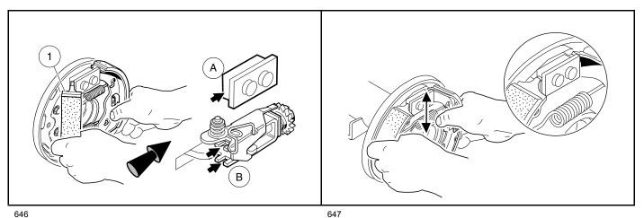
Figure 6-14 Install Leading Shoe
