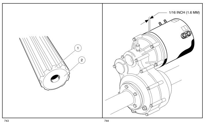
Figure 16-23 Clean Chamfer and Input Shaft End
