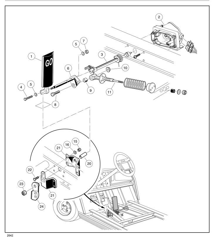
Figure 5-8 Accelerator Pedal – Electric Vehicle with MCOR
