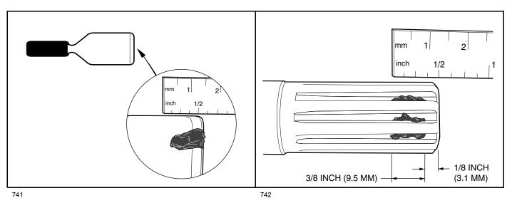
Figure 16-21 Grease on Putty Knife
