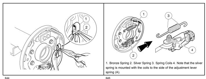
Figure 6-12 Install Trailing Shoe Retainer Clip
