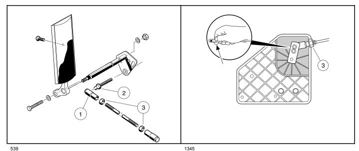
Figure 23-4 Accelerator Rod
