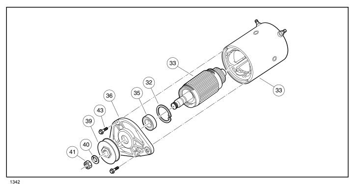
Figure 20-6 Output End Cover Assembly, Armature and Housing
