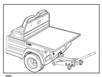
Figure 9-2 Lifting Position
