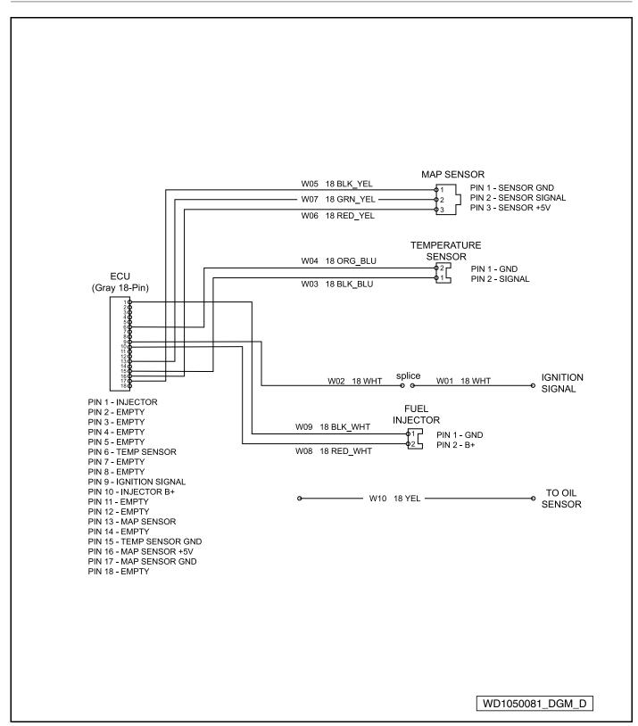
Figure 18-4 Wiring Diagram – EFI and Engine
