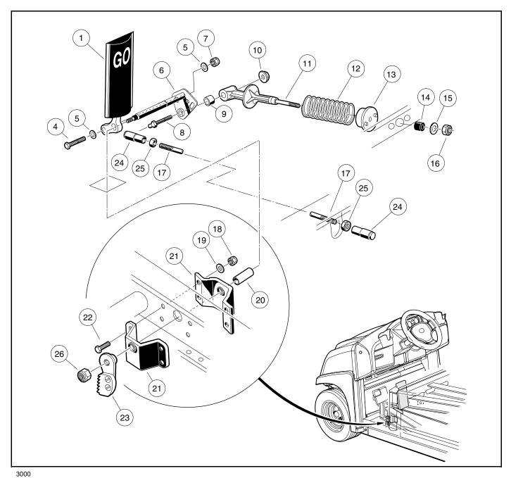
Figure 5-6 Accelerator Pedal – Gasoline Vehicles
