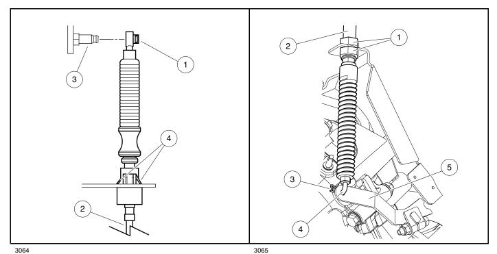
Figure 26-13 Shifter Cable at FNR Handle
