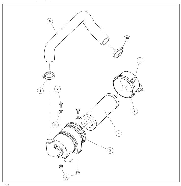
Figure 23-12 Air Intake System – CA 300
