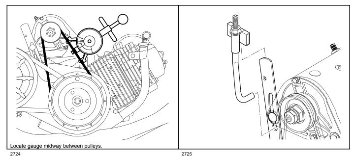
Figure 20-15 Belt Tension Gauge
