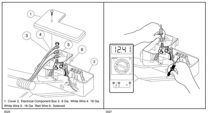
Figure 19-5 Solenoid Wire Removal
