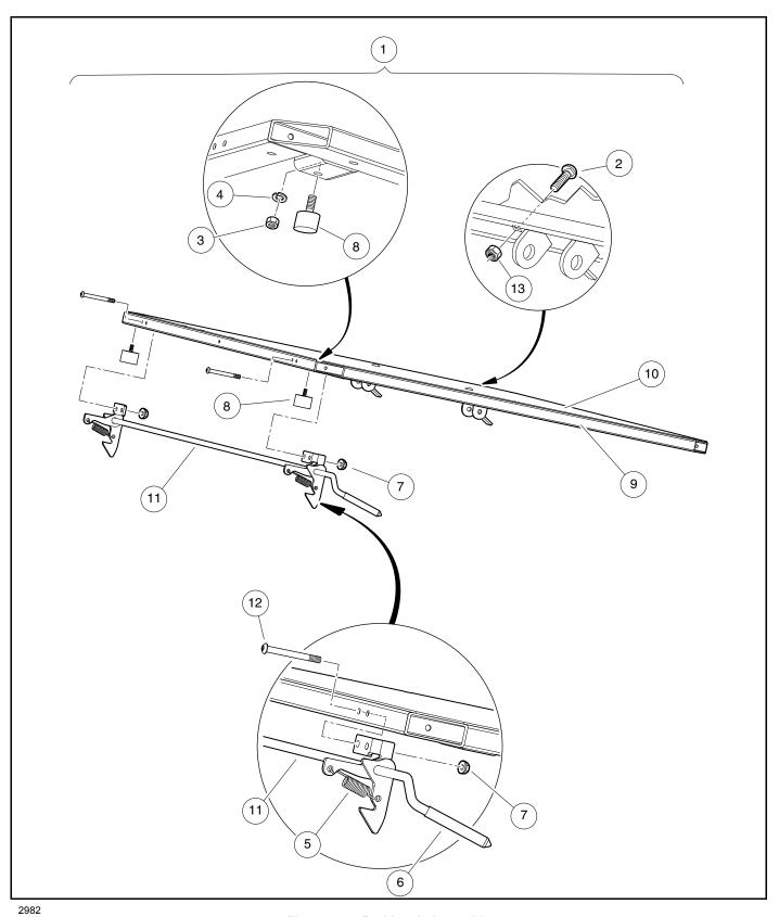
Figure 4-7 Bed Latch Assembly
