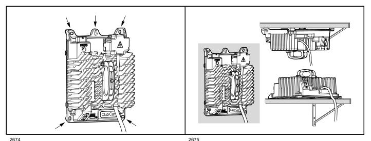
Figure 15-2 Charger Mounting Holes
