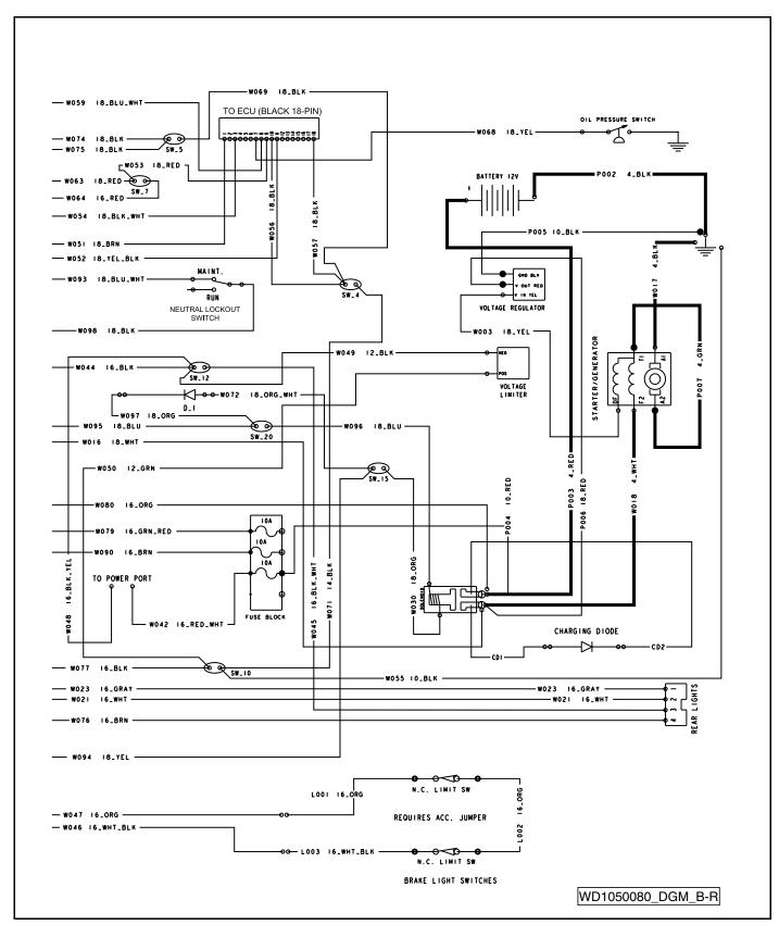
Figure 19-2 Wiring Diagram for Key-Start Gasoline Vehicle - Continued
