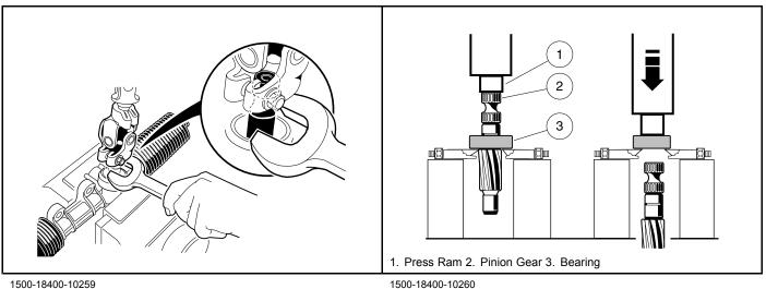
Figure 7-7 Remove Pinion from Housing
