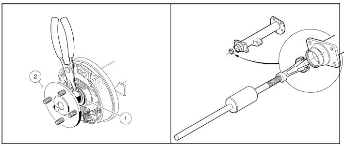
Figure 17-1 Remove Internal Retaining Ring
