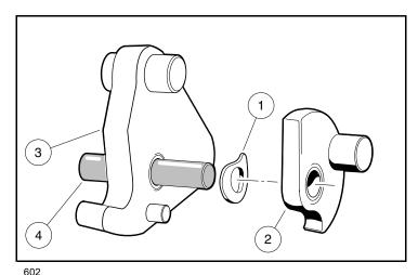
Figure 25-10 Primary and Secondary Weights, Wave Washer and Pin
