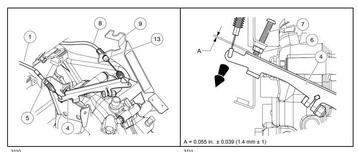
Figure 23-8 Governor and Accelerator Cables At Governor Arm
