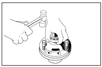
Figure 17-14 Separate Housing
