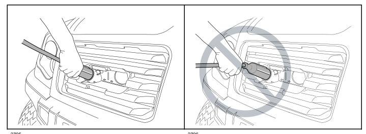
Figure 15-6 Correct Insertion of External Charger DC Plug
