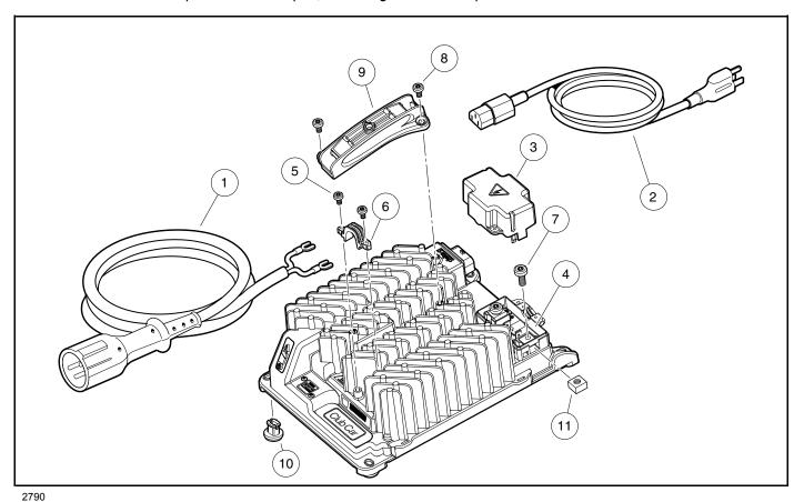
Figure 15-8 External High-Frequency Charger Components
