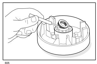
Figure 25-11 Spiral Back-up Rings
