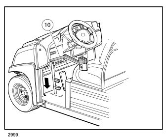
Figure 5-2 Brake Pedal Weldment Through Floor
