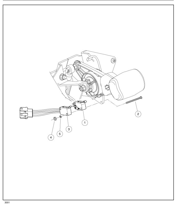
Figure 20-22 Forward/Reverse Assembly Switches
