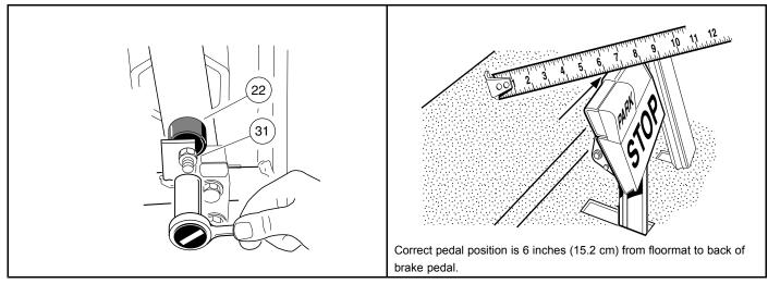
Figure 5-10 Brake Pedal Height Adjustment
