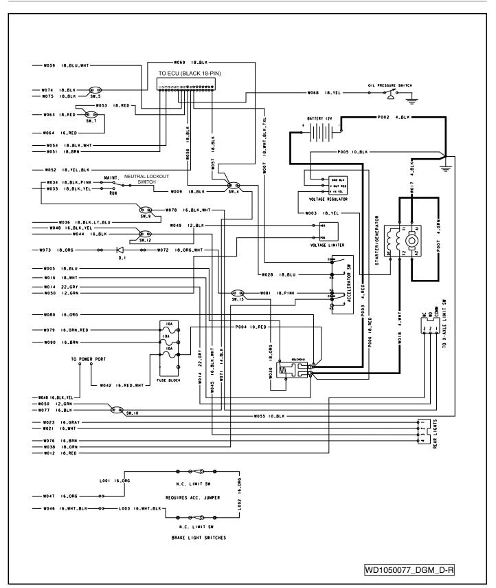
Figure 18-2 Wiring Diagram for Pedal-Start Gasoline Vehicle - Continued
