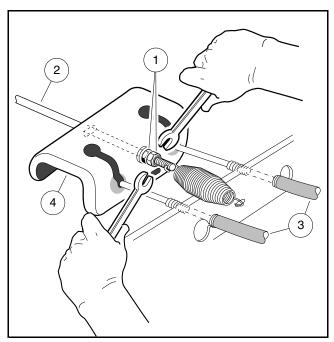
Figure 5-9 Loosen Rear Brake Equalizer Rod Nuts
