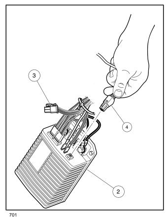
Figure 11-3 Disconnect Four-pin Connector.
