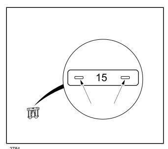
Figure 18-6 Testing the ATC and ATM-style Blade Fuse
