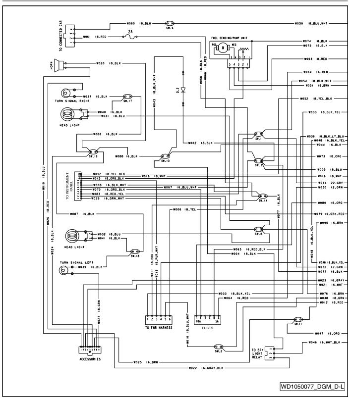
Figure 18-1 Wiring Diagram for Pedal-Start Gasoline Vehicle
