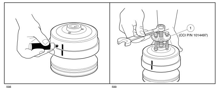
Figure 25-6 Mark Drive Clutch Hub
