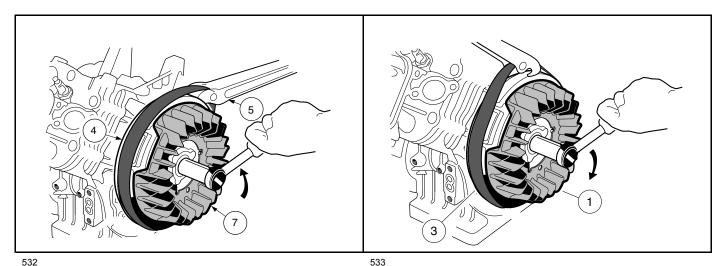
Figure 22-9 Flywheel Nut Removal
