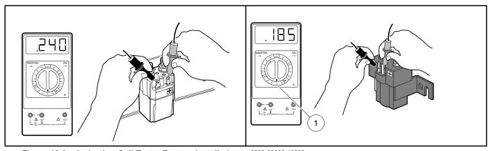
Figure 12-9 Activating Coil Test – Factory-installed Solenoid
