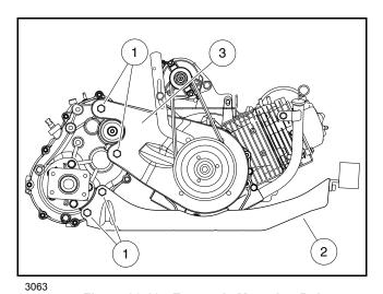
Figure 26-12 Transaxle Mounting Bolts
