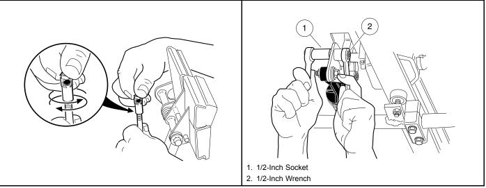
Figure 5-25 Brake Rod Adjustment
