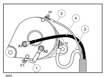
Figure 20-14 Starter/Generator Wiring
