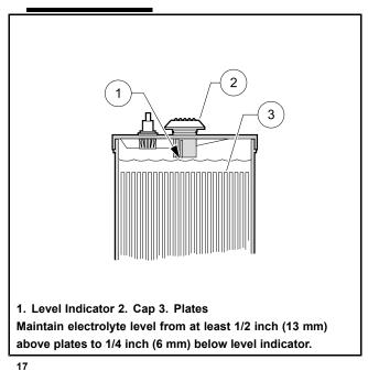
Figure 14-4 Electric Battery Electrolyte Level
