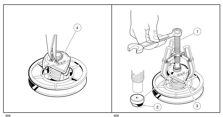
Figure 25-15 Remove Retaining Ring
