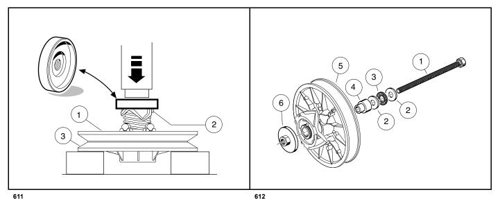
Figure 25-17 Cam Press Tool
