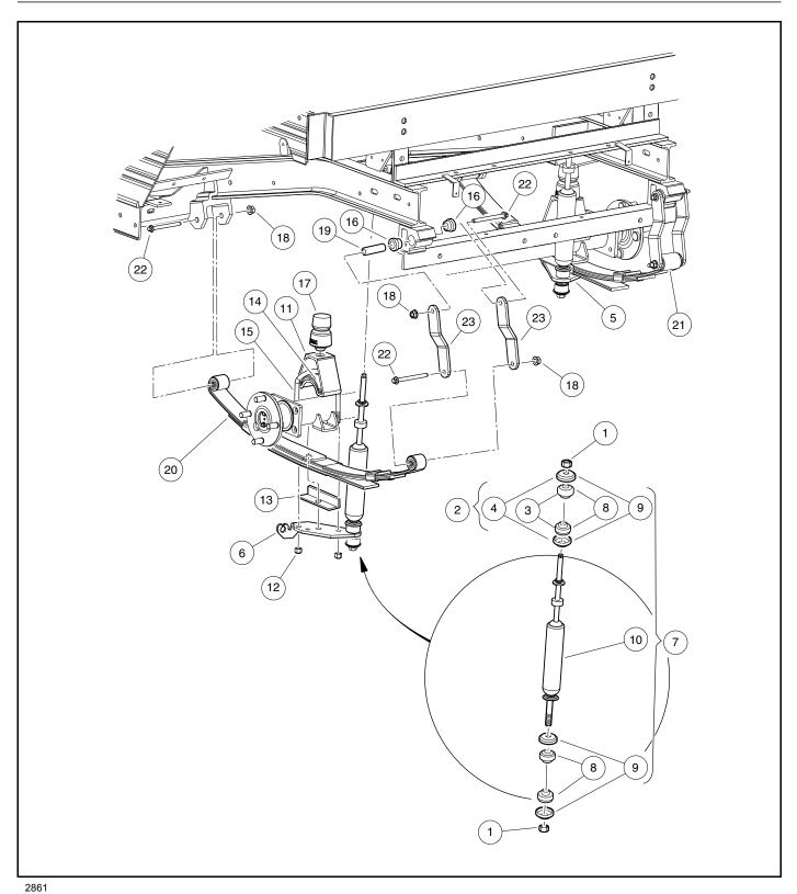
Figure 9-5 Rear Suspension Assembly and Mounting
