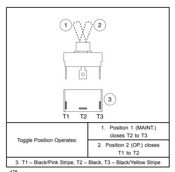
Figure 18-11 Maintenance/Operate Switch Test – for Pedal-Start Vehicles
